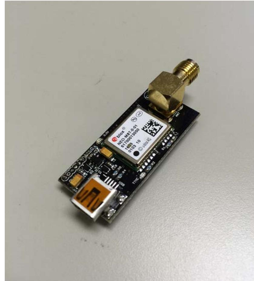
UBLOX NEO-M8T TIME & RAW receiver board with SMA (RTK ready)
